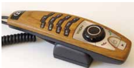
Finished phone prototype with wood, ABS and aluminum parts milled by the MDX-540.
